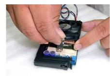
Attaching the heatsink/fan's retaining clip to the ZIF socket. (1)
